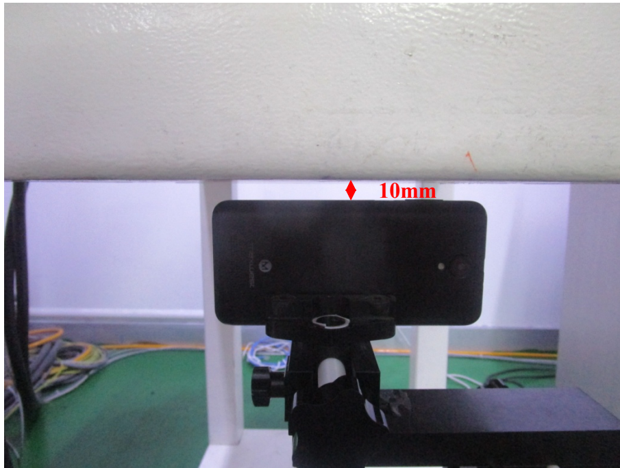
Body Right Setup Photo (10mm)
