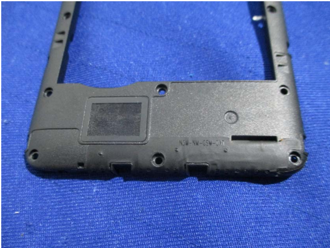
GSM&WCDMA&LTE MAIN Antenna View
