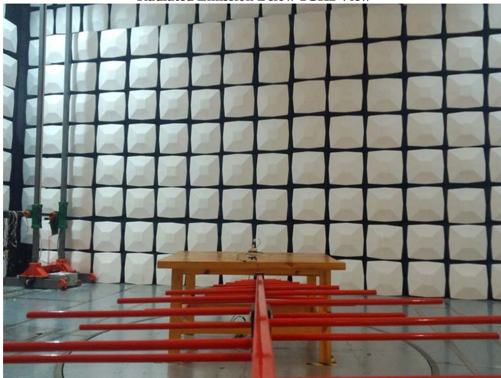
Radiated Emission Below 1GHz View
