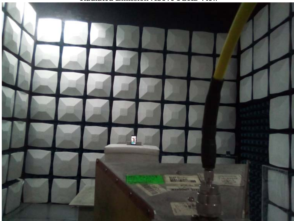
Radiated Emission Above 1GHz View
