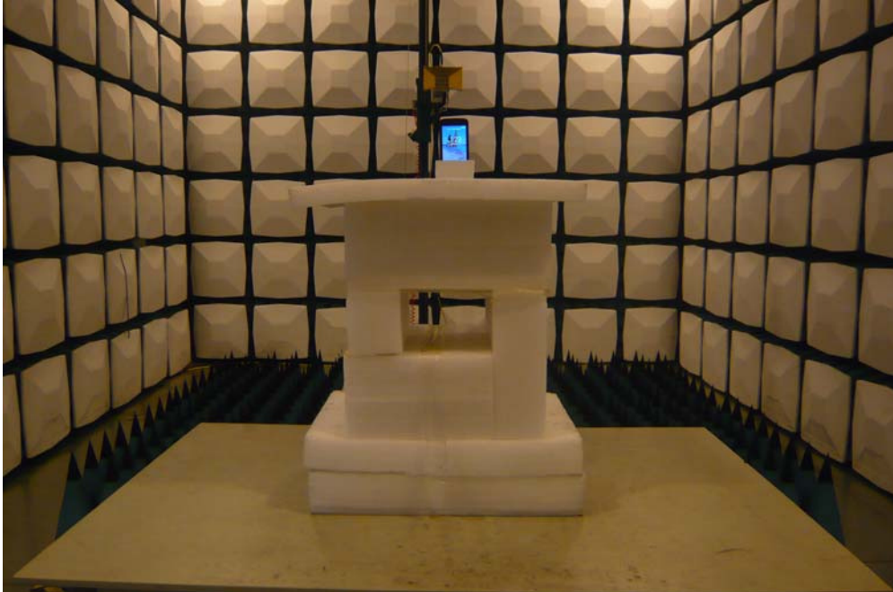
Radiated Emission View (Above 1GHz)
