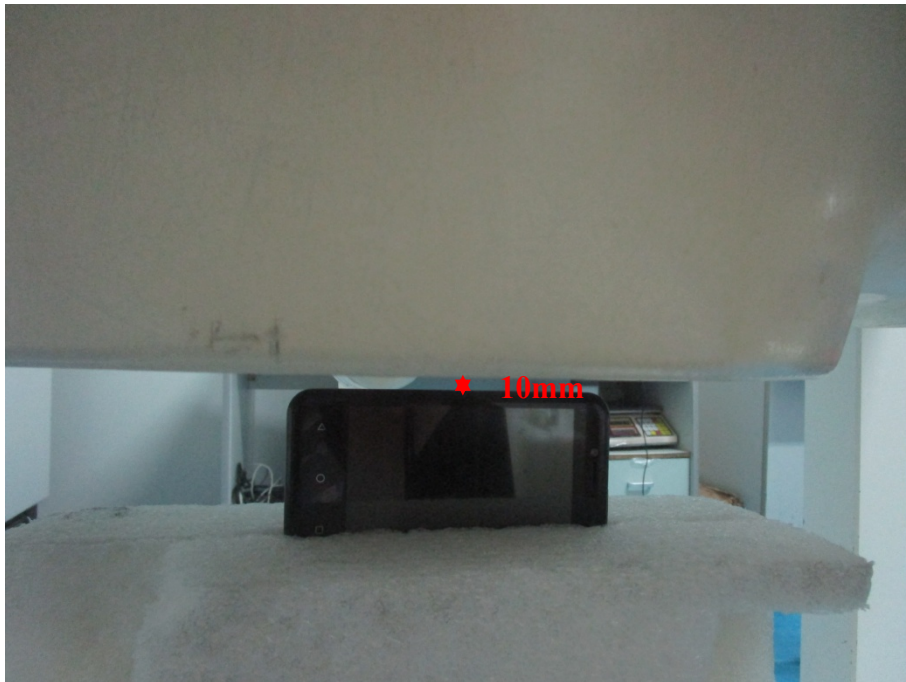
Body Left Setup Photo(10mm)
