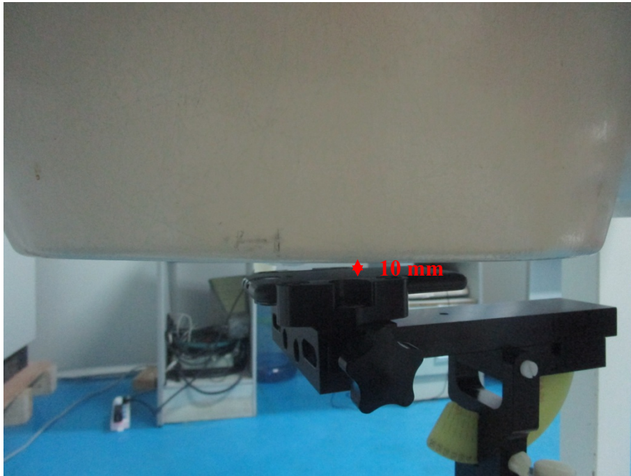
Body Left Setup Photo(10mm)
