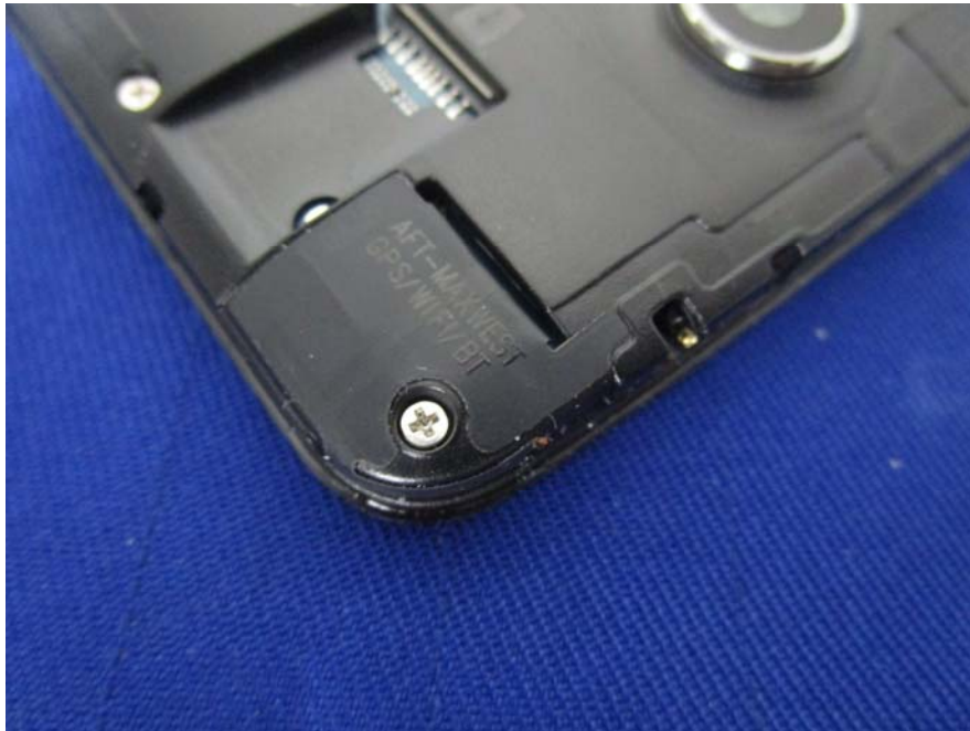
EUT – BT&wifi Antenna View
