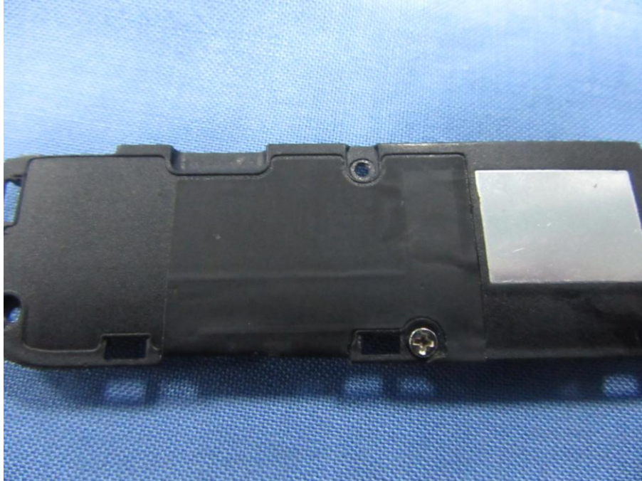
EUT – GSM&WCDMA Antenna View
