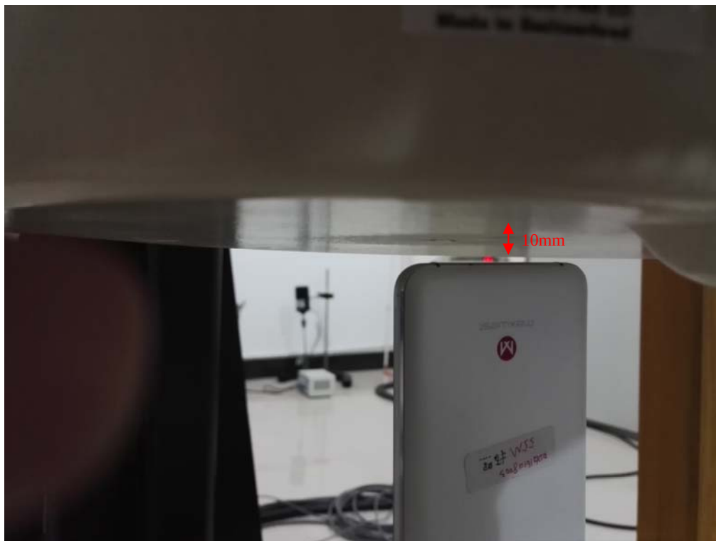
Body-worn Bottom Setup Photo (10mm)
