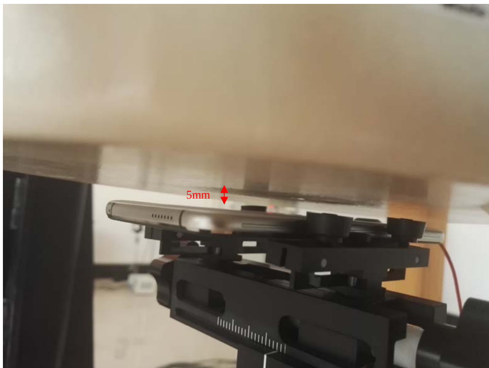
Body-worn- Back Setup Photo (5mm)
