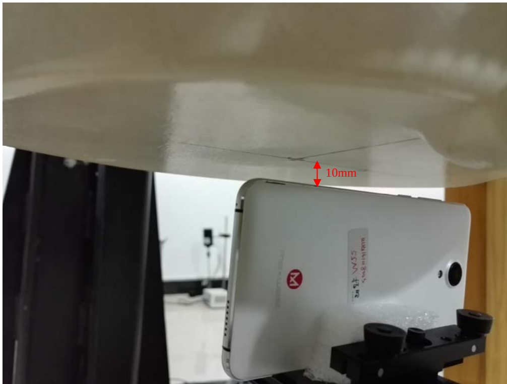
Body-worn Bottom Setup Photo (10mm)
