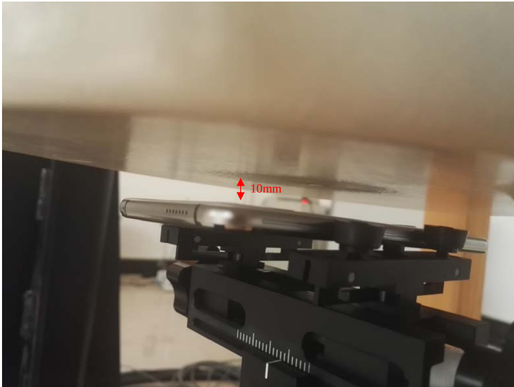
Body-worn Back Setup Photo (10mm)
