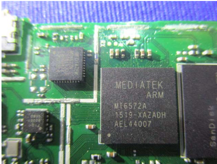
EUT –Main Chip View
