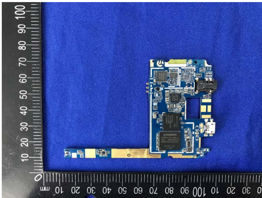
EUT –Main Board Bottom Unshielded View
