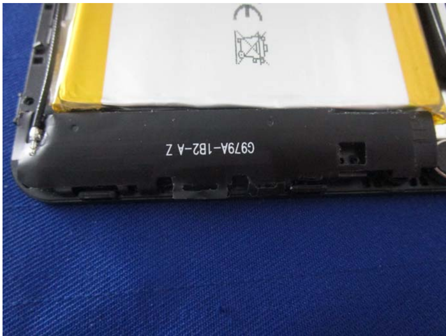
EUT – LTE&2G&3G Antenna View
