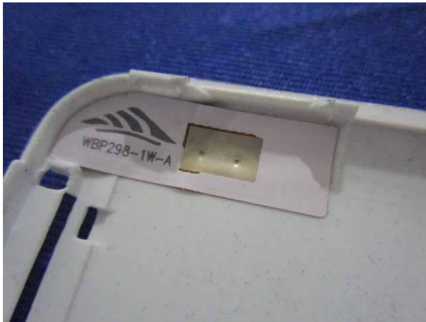
EUT –Wifi &BT Antenna View
