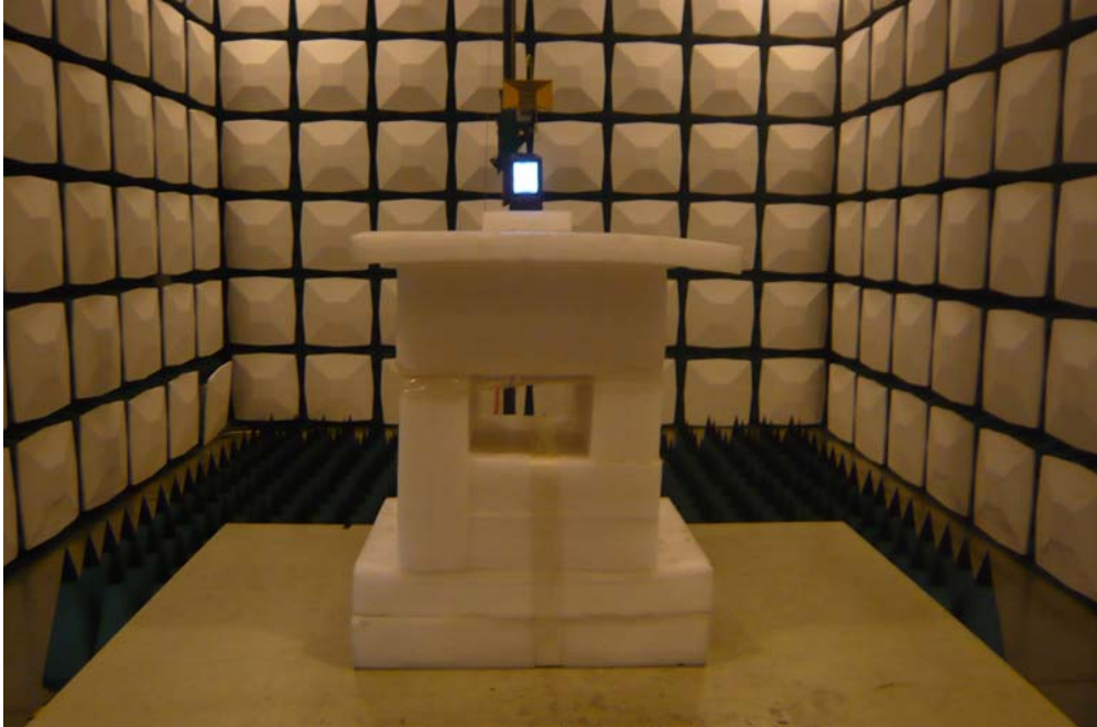
Radiated Emission View (Above 1GHz)
