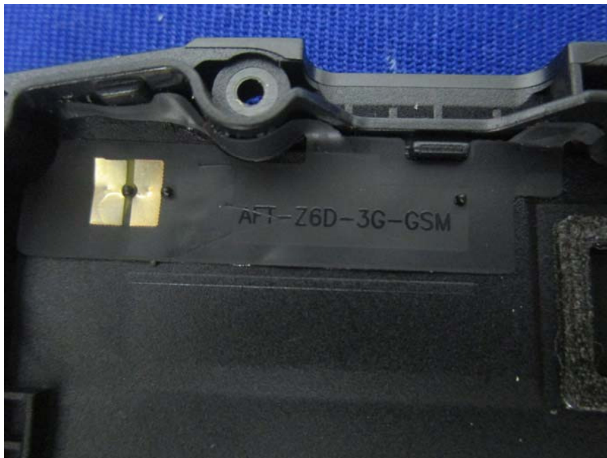
EUT – GSM Antenna View
