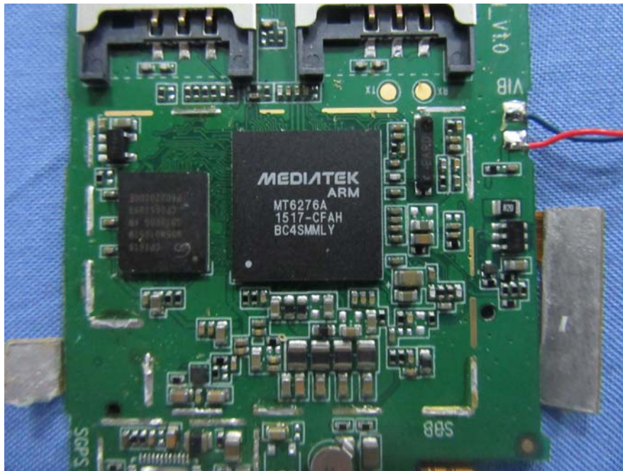
EUT – Bluetooth Chip View
