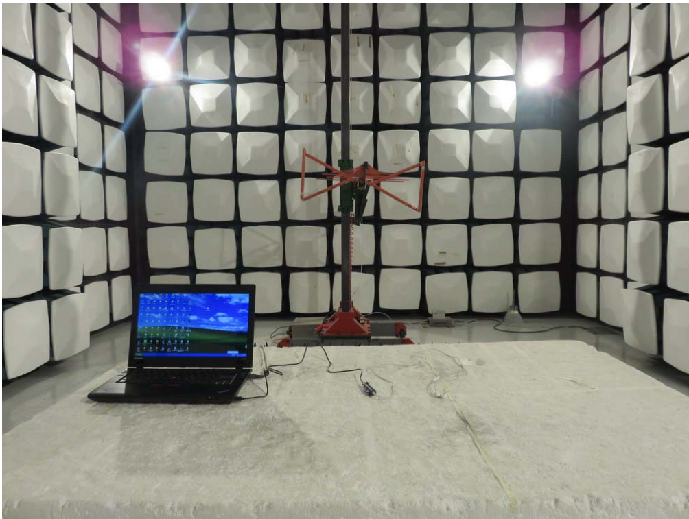
FCC RADIATED EMISSION TEST SETUP
