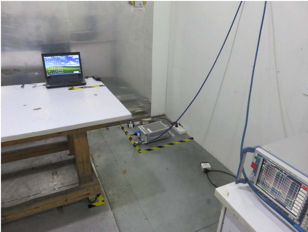
FCC RADIATED EMISSION TEST SETUP
