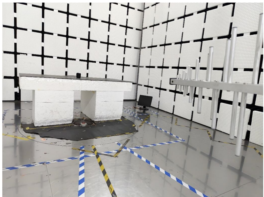
Radiation Emission Test Setup (30MHz to 1GHz)
