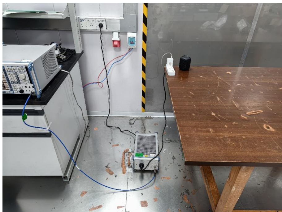
Conducted Emission Test Setup
