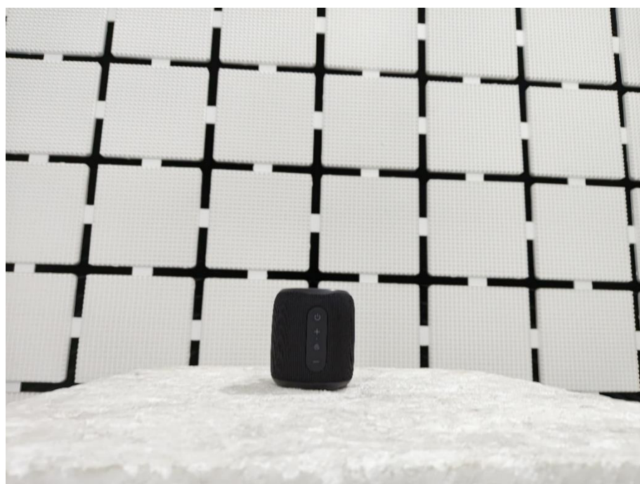
Radiation Emission Test Setup (close up)
