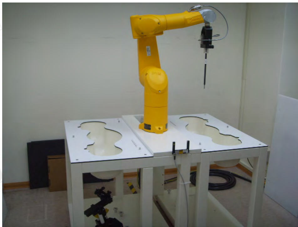
Fig.1 Photograph of the SAR measurement system
