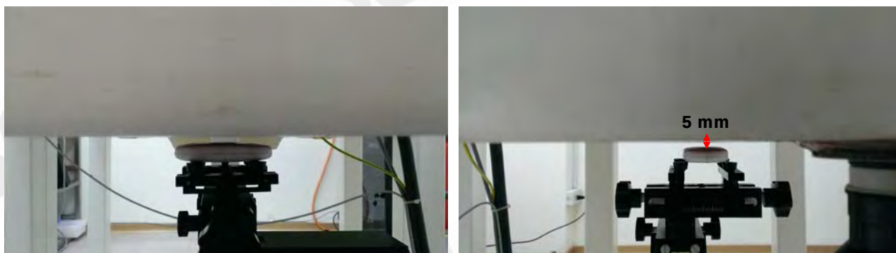
Fig.3 EUT front side to flat phantom
