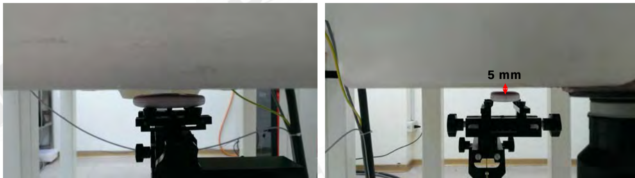
Fig.3 EUT front side to flat phantom
