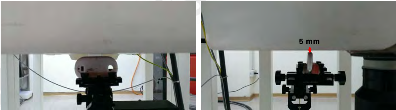
Fig.6 EUT bottom side to flat phantom
