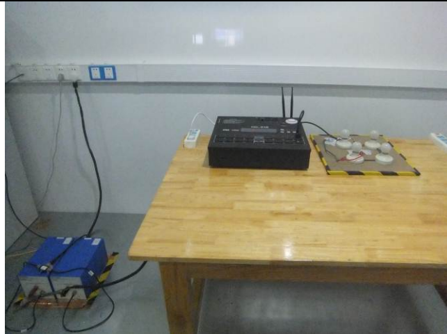
Conducted Emissions Test Setup Front View
