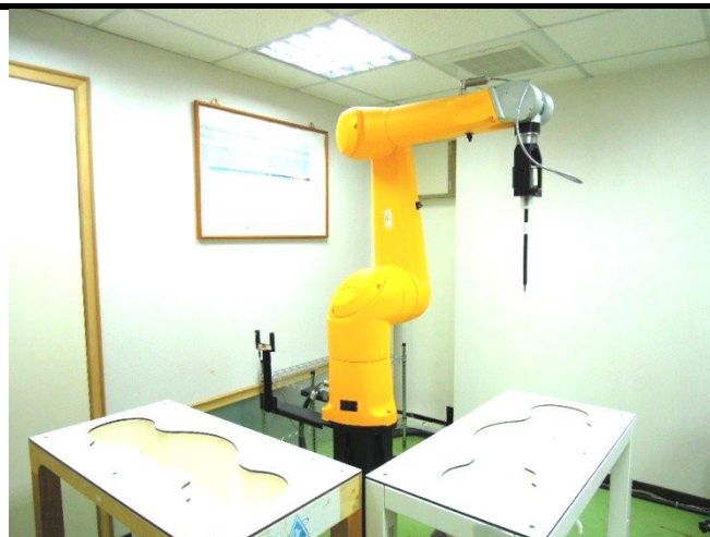
Fig-3.2 SPEAG DASY52 System
