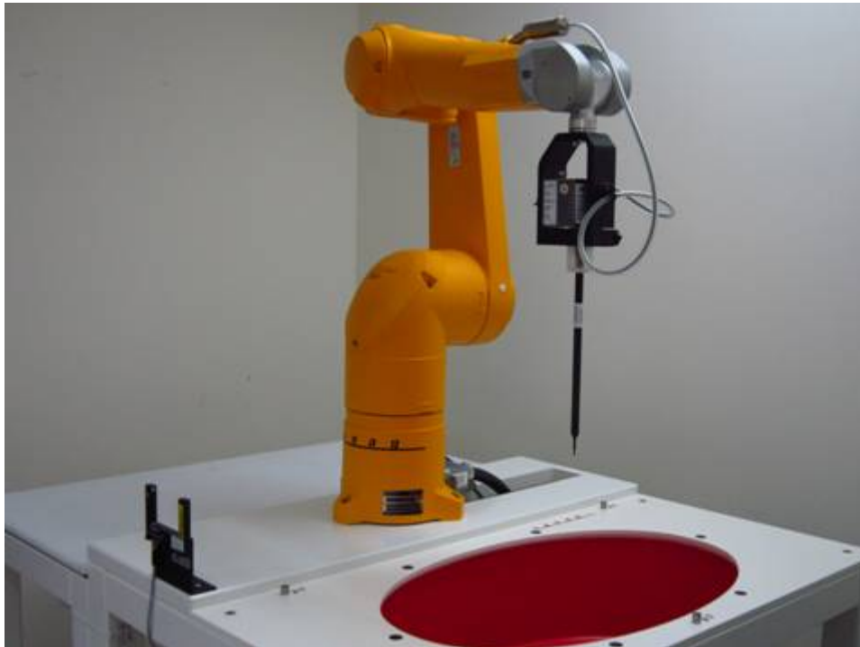
Fig.1 Photograph of the SAR measurement system
