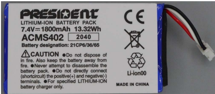
Figure E18.10 – Internal Photo – Battery
