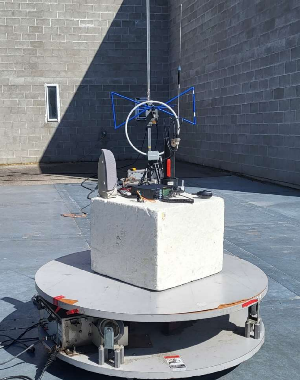
Figure E18.4 – Setup, Radiated Emissions Below 30MHz, with Accessories
