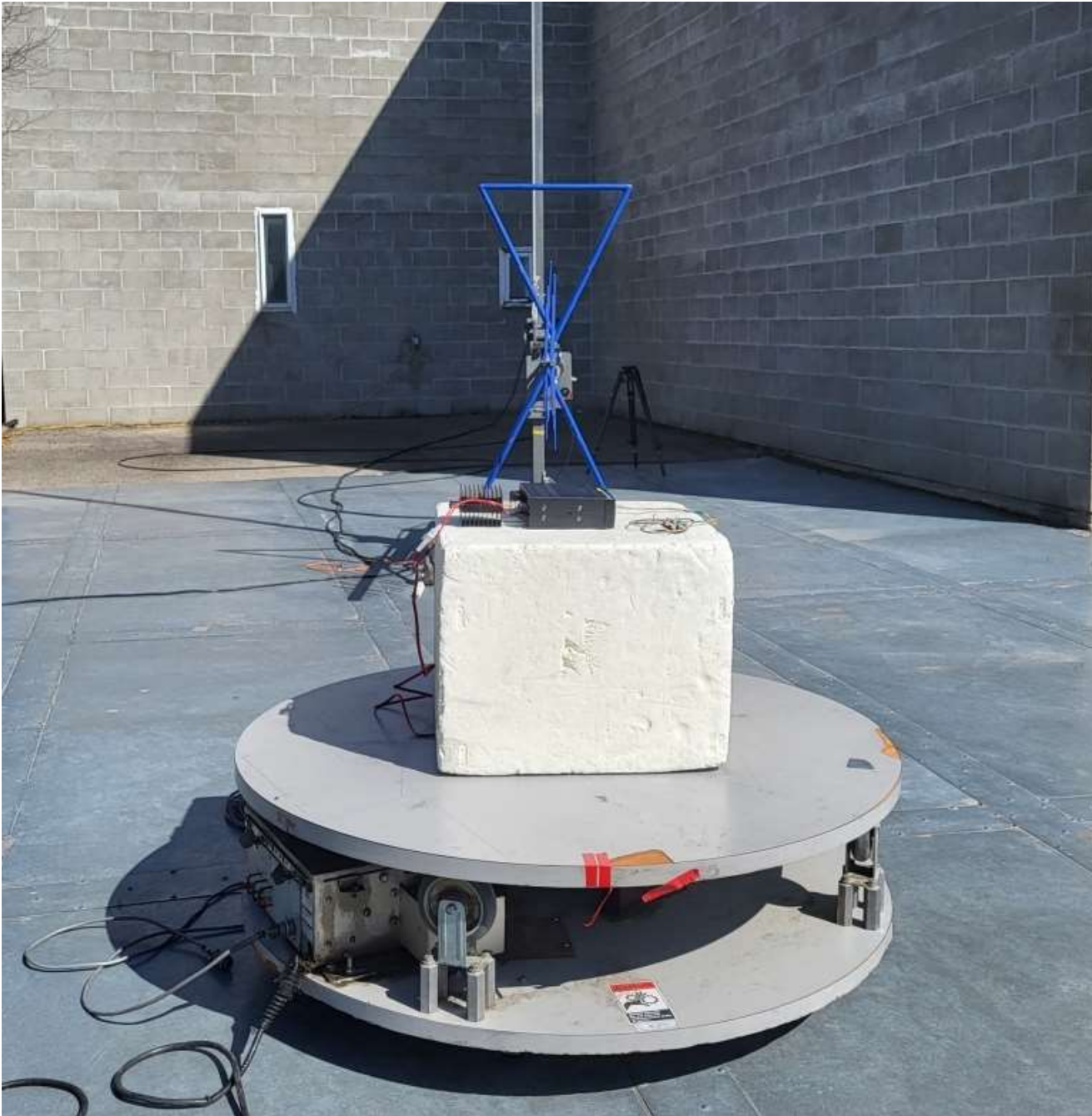
Figure E18.7 – Setup, Radiated Emissions 30 - 1000MHz, without Accessories
