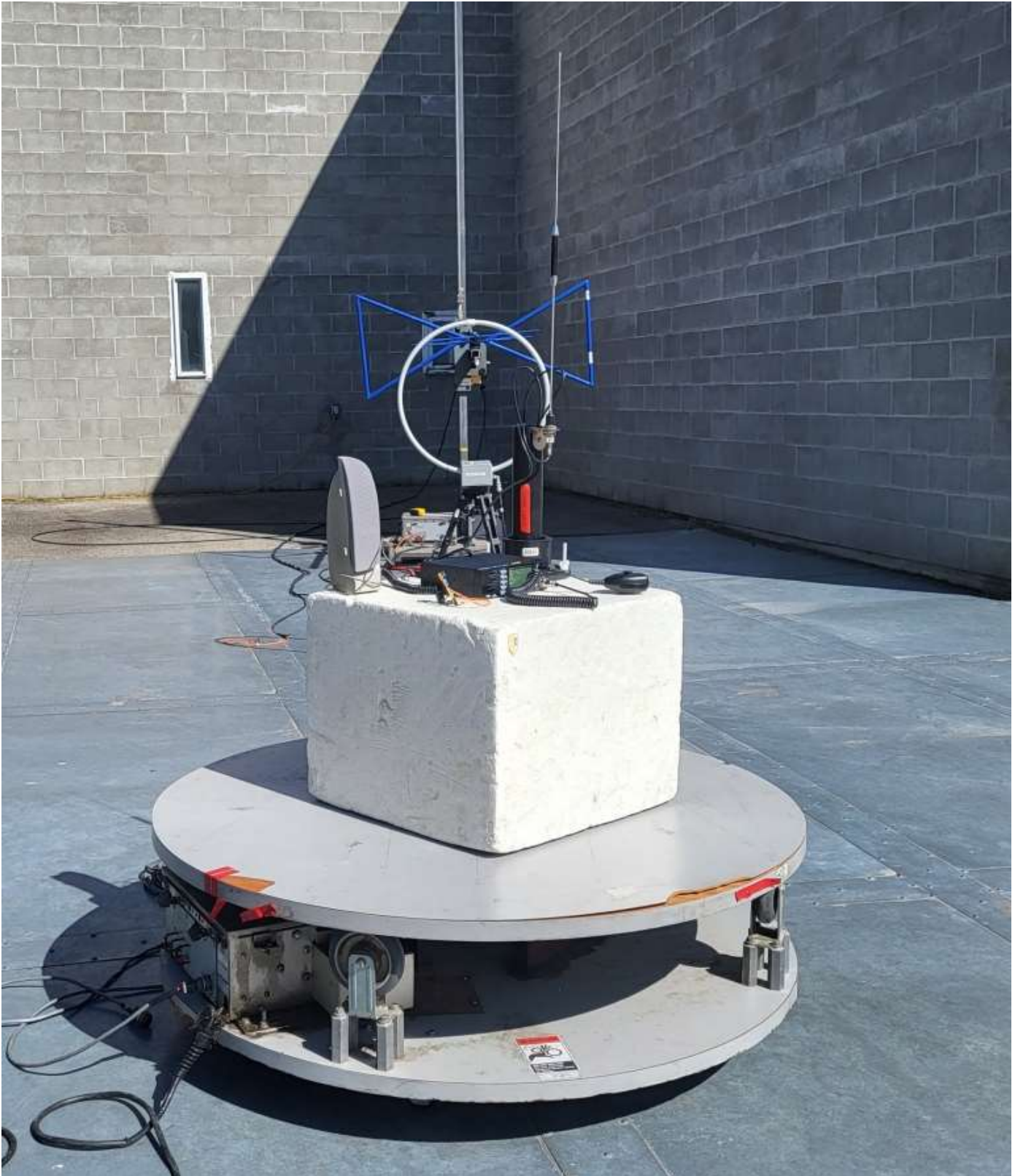
Figure E18.8 – Setup, Radiated Emissions 30 - 1000MHz, with Accessories
