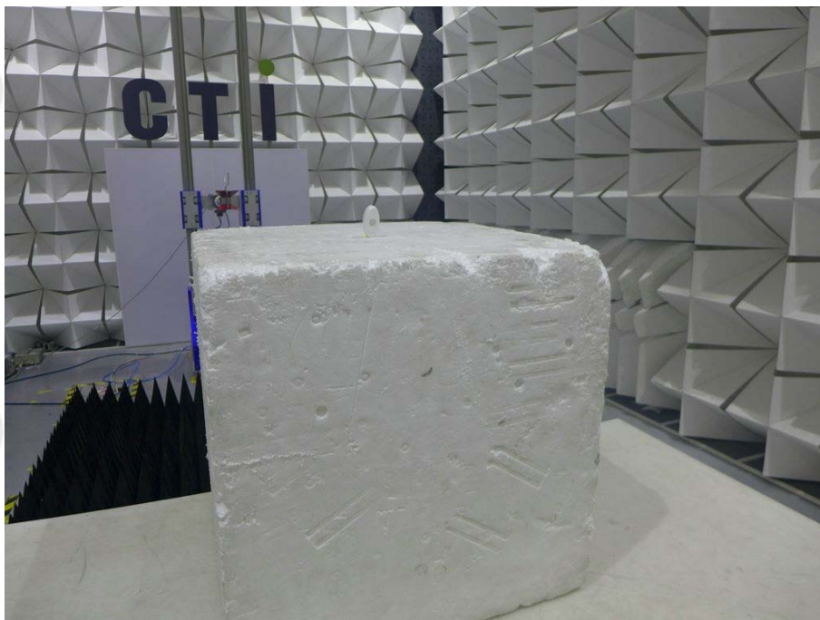
Radiated spurious emission Test Setup for 2324TX -3(Above 1GHz)
