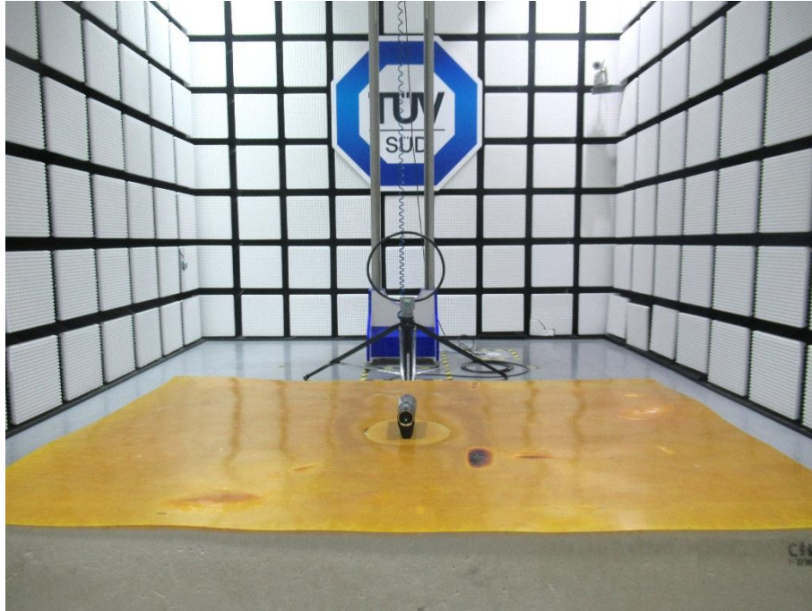
9kHz-30MHz RSE Setup
