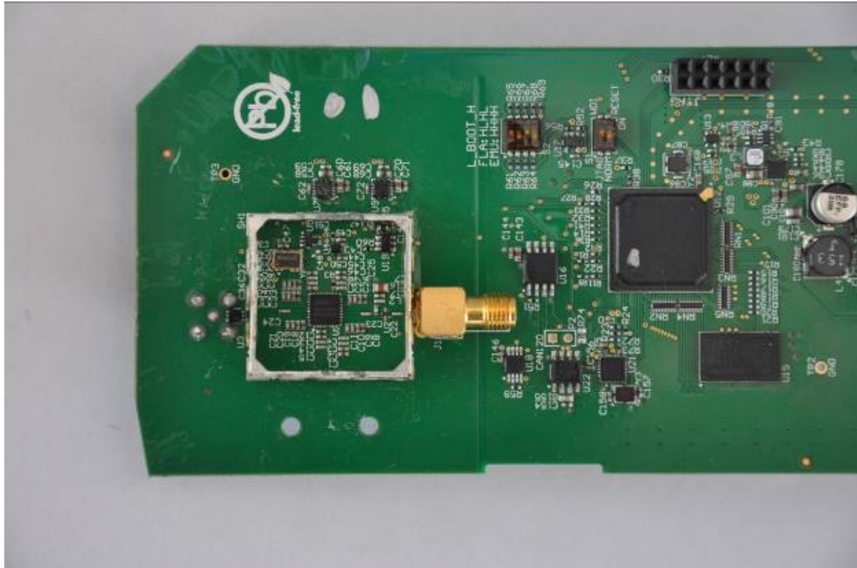
Figure 8. RF Module with Shield Removed
