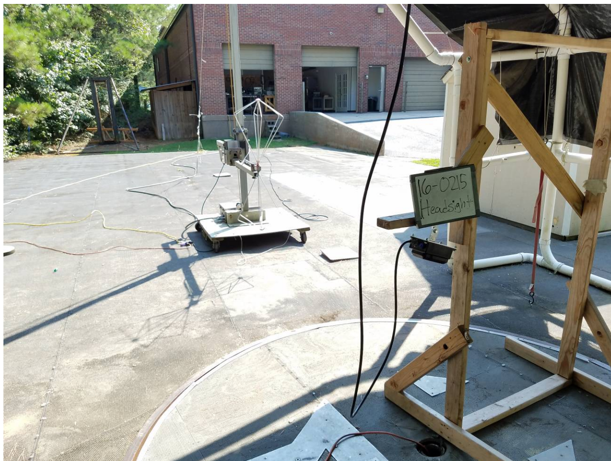
Figure 1. Radiated Emissions Test Setup, 30 MHz to 200 MHz, Single Config
