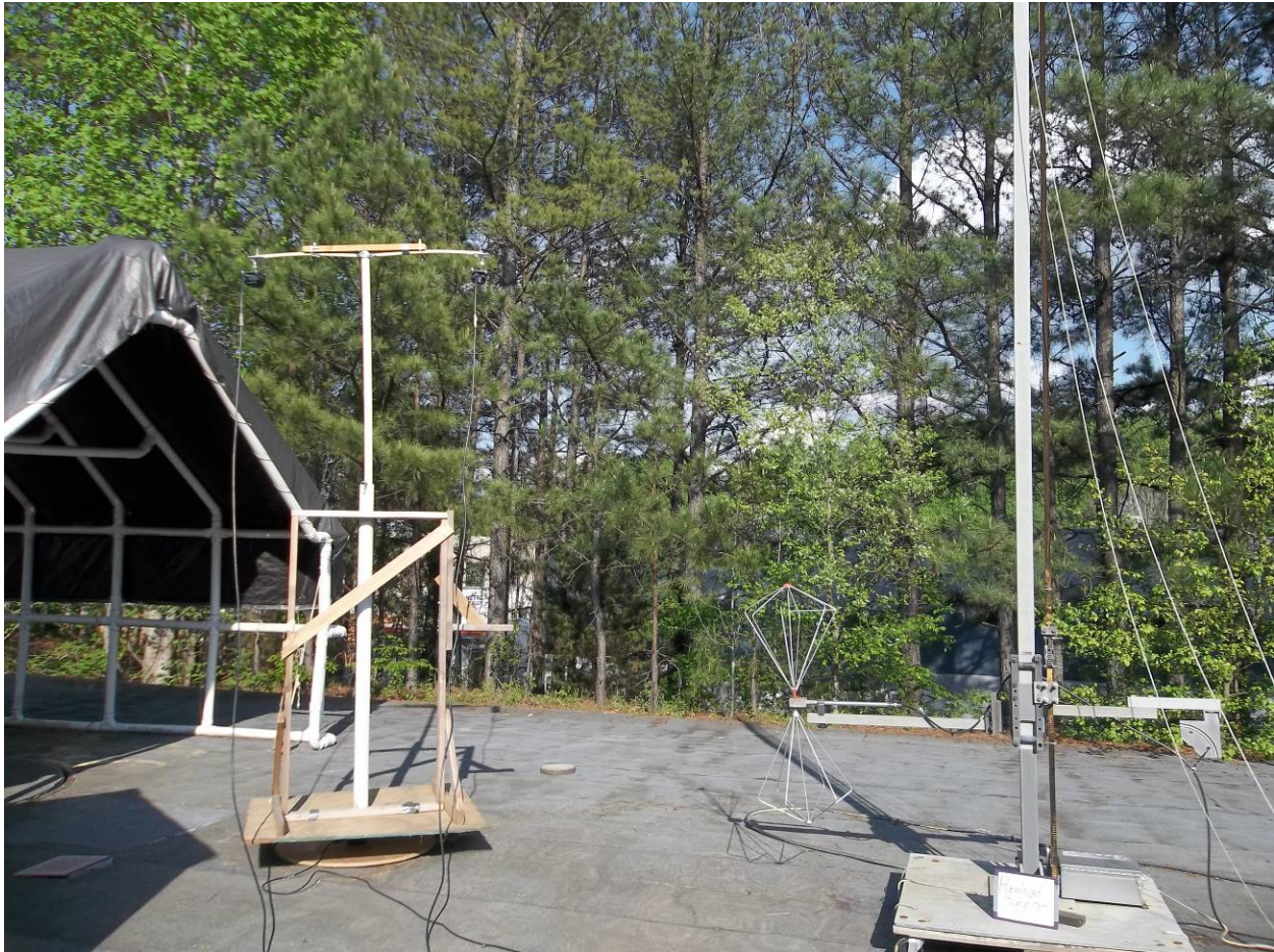
Figure 2. Radiated Emissions Test Setup, 30 MHz to 200 MHz, Dual Config
