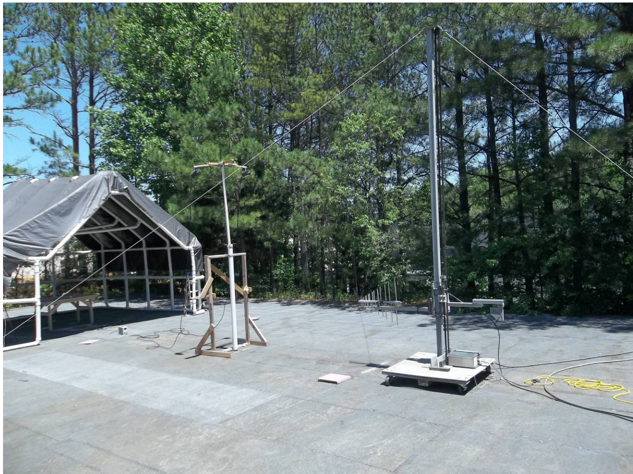
Figure 4. Radiated Emissions Test Setup, 200 MHz to 1GHz, Dual Config
