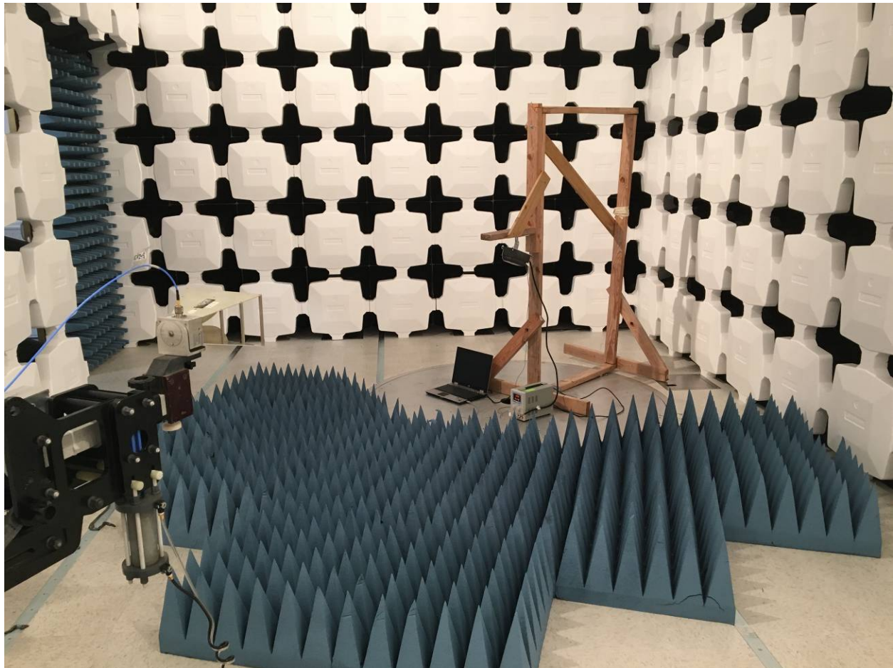
Figure 5. Radiated Emission Test Setup, above 1 GHz, Single Config
