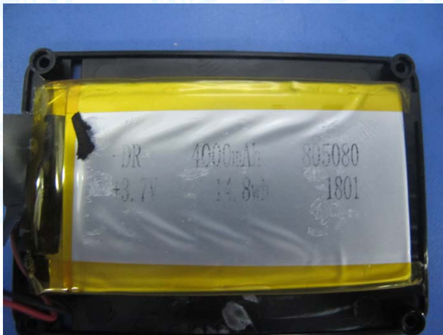
Photo 13 Appearance of Battery
