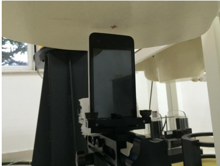
10mm Body-worn Bottom Side Setup Photo
