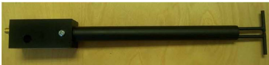
Figure 1 – MVG COMOSAR Validation Dipole
