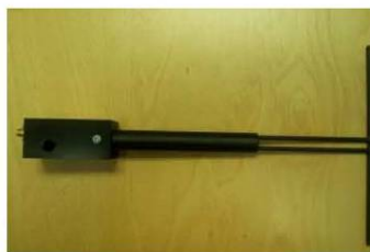
Figure 1 – MVG COMOSAR Validation Dipole
