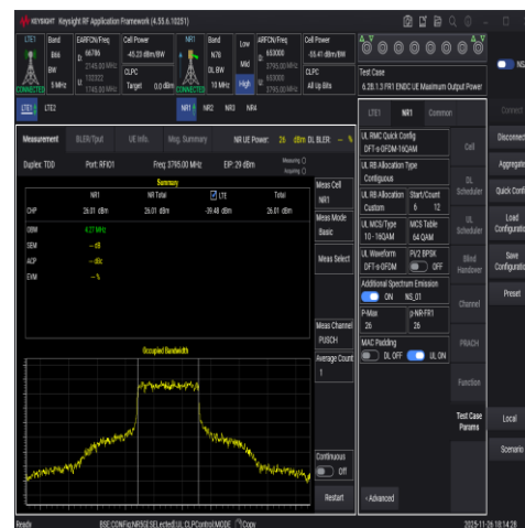
NTNV-DC_66A_n78A-3700-3800-PC2-30-5+10-M +H-N/A-N/A-DFT-16QAM-Inner Full-PASS
