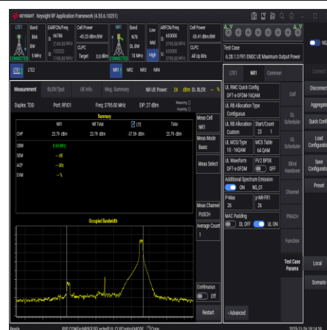
NTNV-DC_66A_n78A-3700-3800-PC2-30-5+10-M +H-N/A-N/A-DFT-16QAM-Edge 1RB Right-PASS
