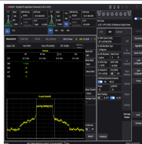
NTNV-DC_66A_n78A-3700-3800-PC2-30-5+15-M +H-N/A-N/A-DFT-QPSK-Inner Full-PASS
