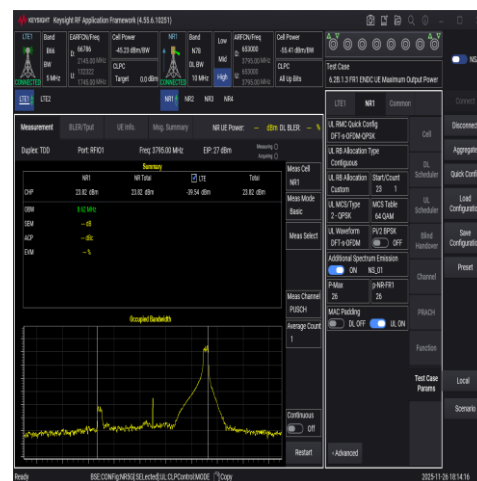
NTNV-DC_66A_n78A-3700-3800-PC2-30-5+10-M +H-N/A-N/A-DFT-QPSK-Edge 1RB Right-PASS
