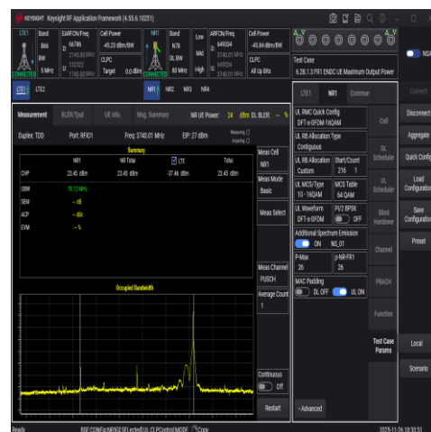
NTNV-DC_66A_n78A-3700-3800-PC2-30-5+80-M +L-N/A-N/A-DFT-16OAM-Edge 1RB Right-PASS
