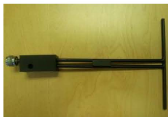
Figure 1 – MVG COMOSAR Validation Dipole
