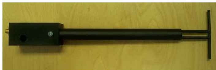
Figure 1 – MVG COMOSAR Validation Dipole
