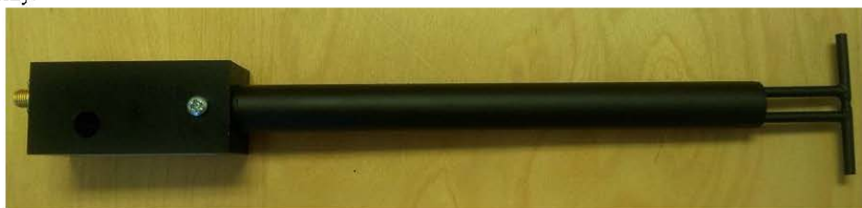
Figure 1 – MVG COMOSAR Validation Dipole
