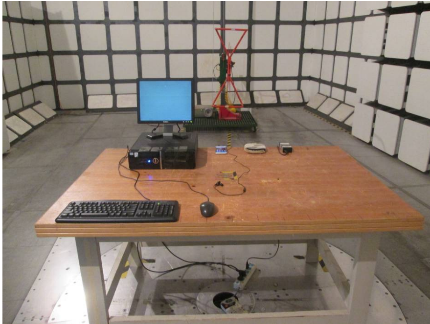
Radiated Emissions – Front View (Below 1 GHz)
