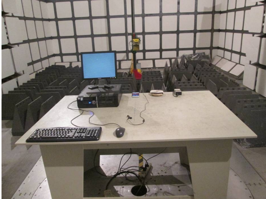
Radiated Emissions – Front View (Above 1 GHz)
