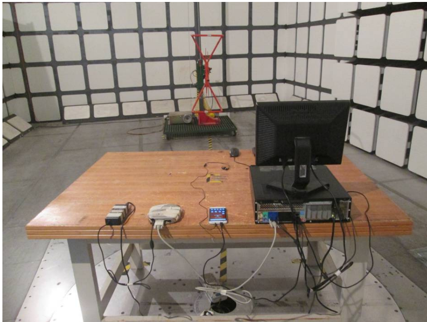
Radiated Emissions – Rear View (Below 1 GHz)
