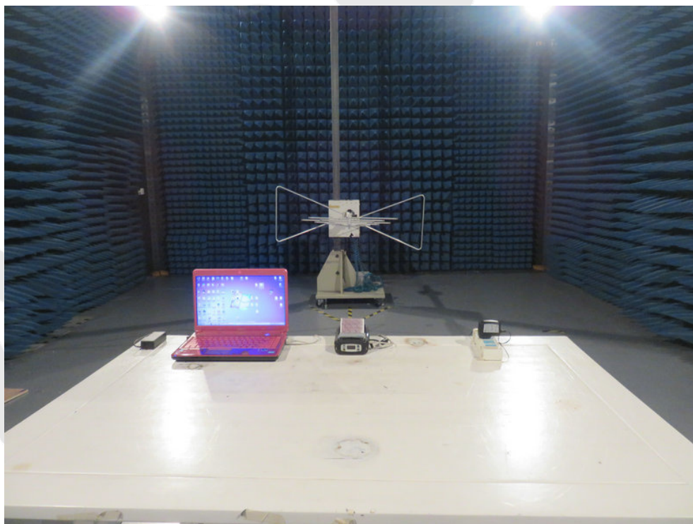
Photo of Radiation Emission Test
