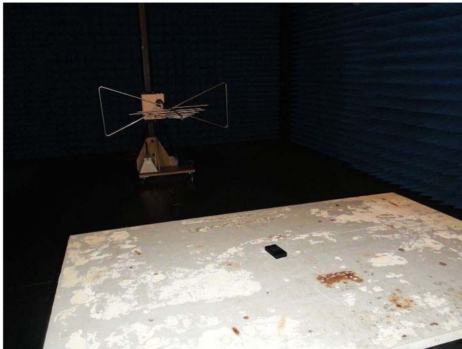
Radiated emission test view
