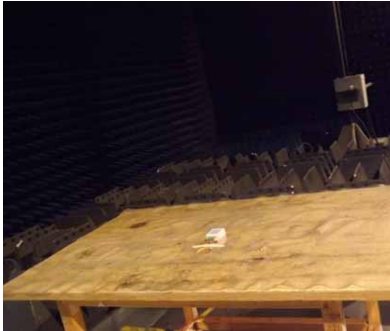
Photograph – Radiated Emission Test Setup for 1GHz ~ 6GHz at Test Site 1#
