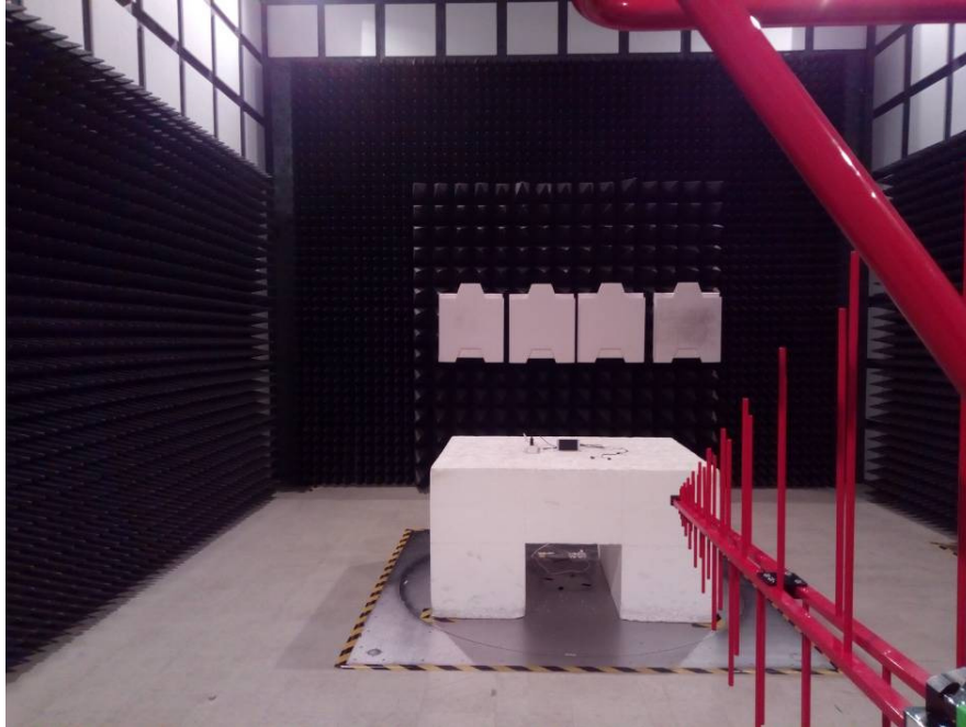
Radiated Emissions View (Below 1 GHz)
