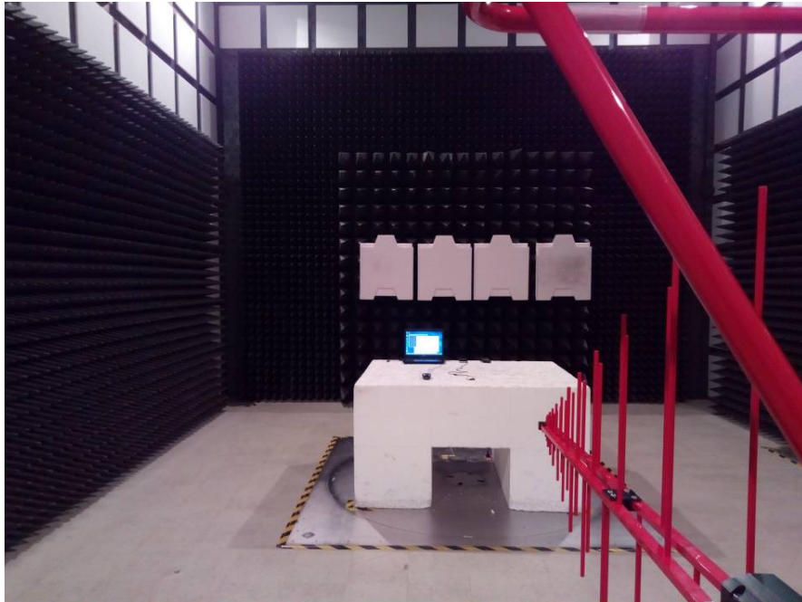
Radiated Emissions – Front View (Below 1 GHz)
