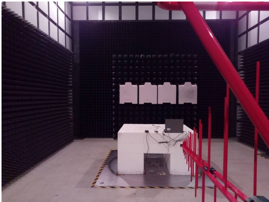
Radiated Emissions – Rear View (Below 1 GHz)
