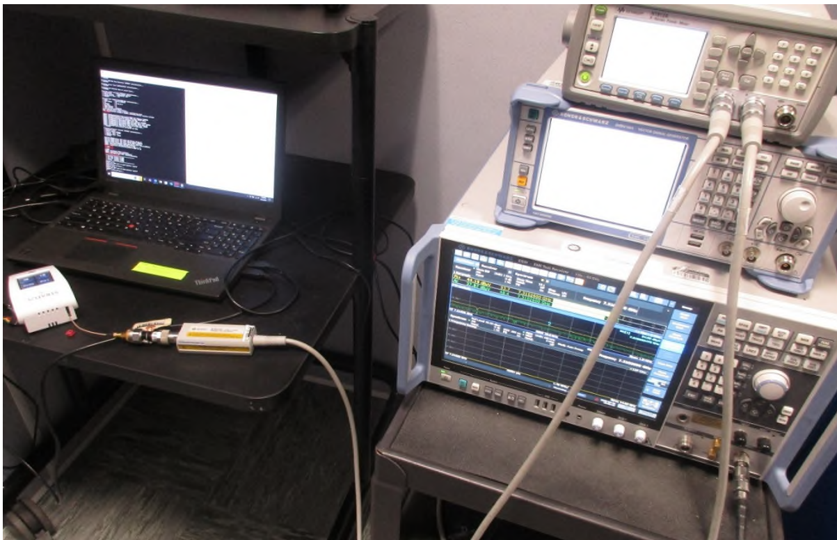
Photo 1.1-1 – Conducted Test Setup
