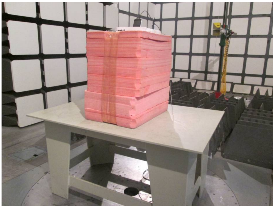
Radiated Emissions View (Above 1 GHz)
