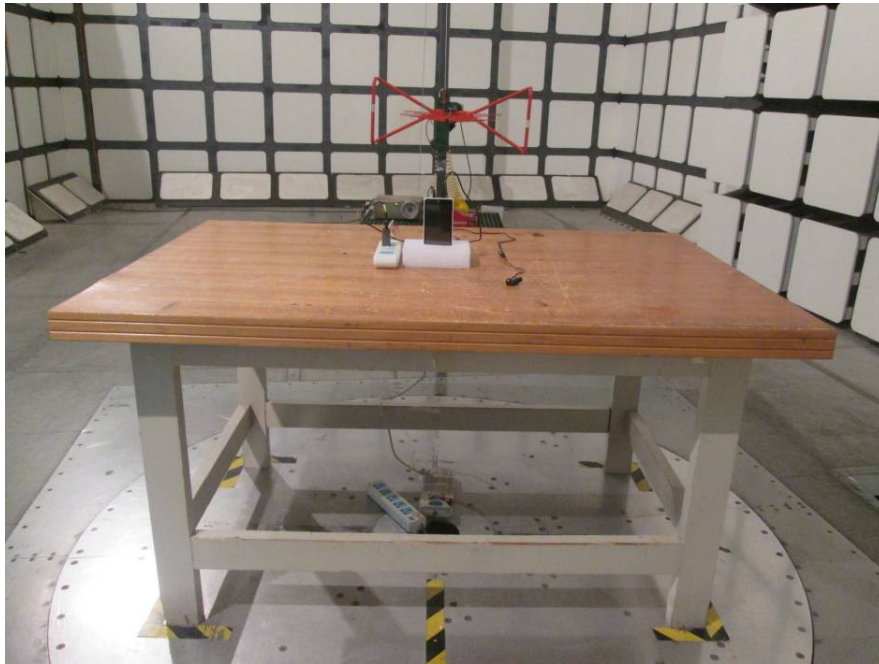
Radiated Emissions View (Below 1 GHz)
