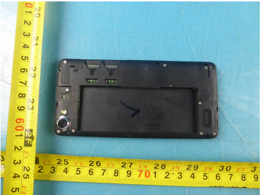
View of internal EUT-2
