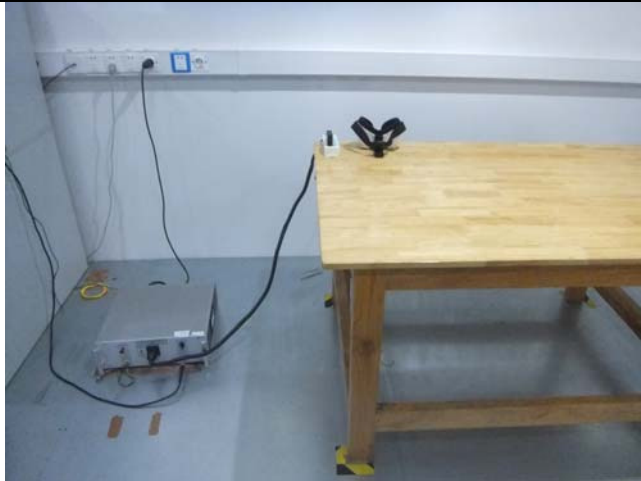
Conducted Emissions Test Setup Front View
