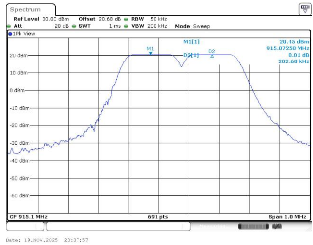
Channel Separation Plot on Channel 915MHz
