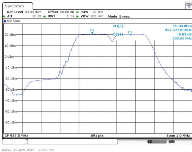
Channel Separation Plot on Channel 927.6MHz
