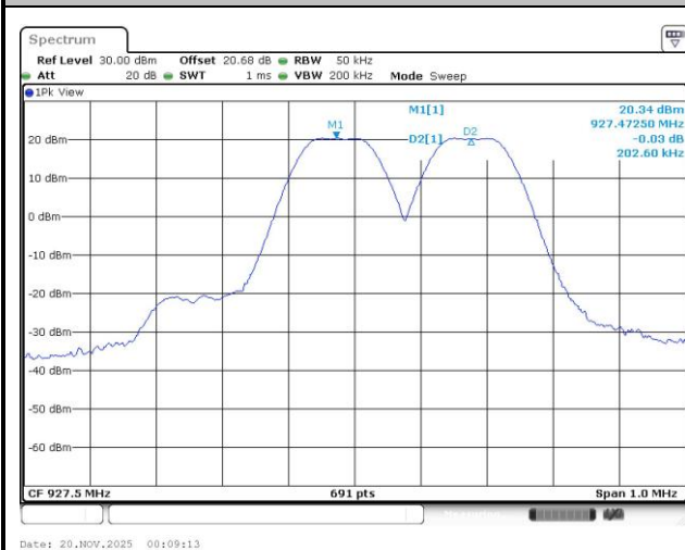
Channel Separation Plot on Channel 927.6MHz
