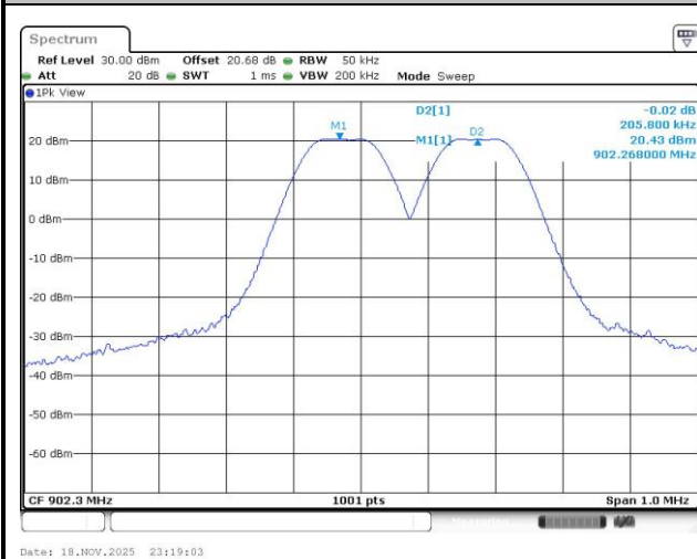
Channel Separation Plot on 902.2MHz
