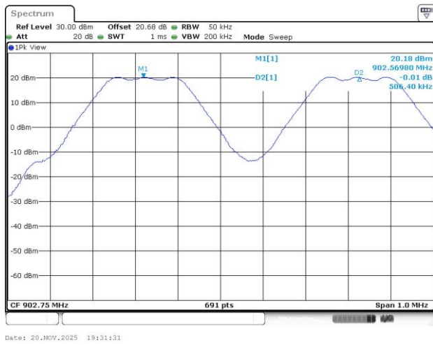
Channel Separation Plot on Channel 927.5MHz
