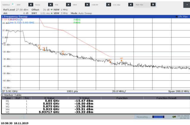
Figure 8.8-18: Conducted emissions at upper band edge measurement, 802.11a
