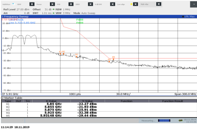
Figure 8.8-19: Conducted emissions at upper band edge measurement, 802.11n
