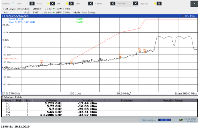
Figure 8.8-17: Conducted emissions at lower band edge measurement, 802.11n
