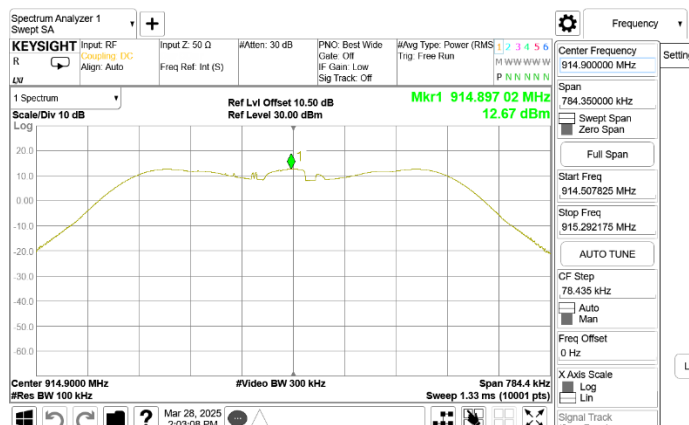
Reference Level _FSK 100Kbps 249bytes_HighCH-926.9MHz
