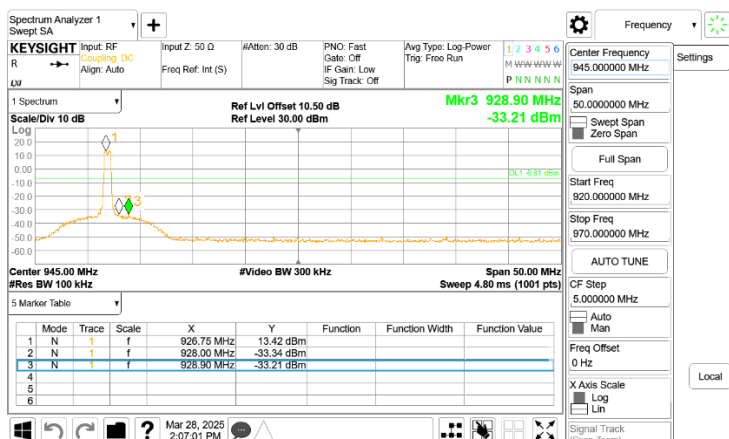
Band Edge _FSK 100Kbps 249bytes_HighCH-926.9MHz
