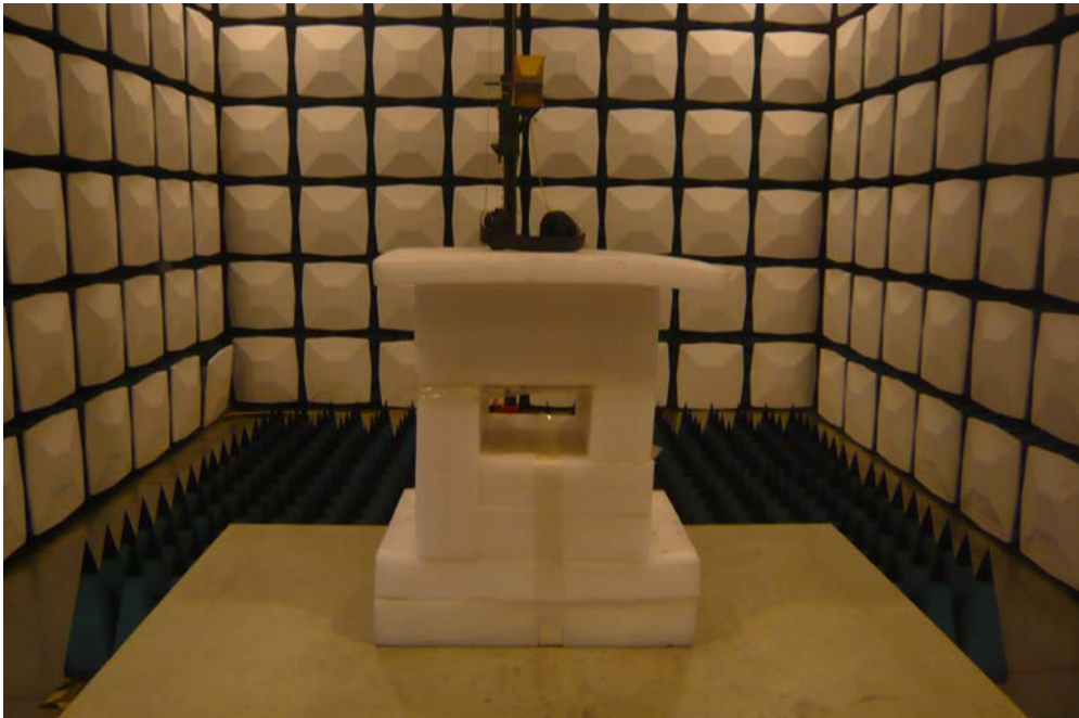
Radiated Emission View (Above 1GHz)
